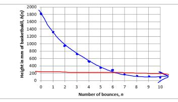
e. Use the curve to estimate the bounce number at which the rebound height will drop below 200 mm.
